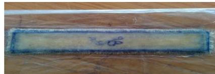
**fig 3.2** Arrangement of mold before curing
